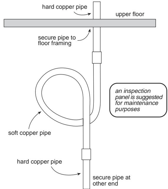
Using a combination of hard and soft copper supply pipe to allow for needed settling in second-story plumbing. The loop of soft pipe opens with settling.
