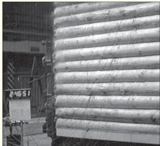
Houdek's experimental log wall. Note the many thermocouple wires to record temperatures inside the wall and on its surface.
